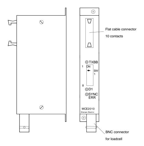
The load cell modules are connected to each other using the supplied cable (10 pole ribbon cable). The MCE2029 analog module is connected using the same cable.
