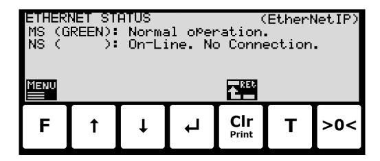
This requires that the EtherNetIP protocol is selected from the menu (the F key) in the ETHERNET STATUS screen. The currently selected protocol is shown in the upper right corner of the screen. If the EtherNetIP protocol is selected, then the EtherNetIP status indications for both Module Status (MS) and Network Status (NS) are shown, corresponding to the normal MS and NS lamps as follows:
