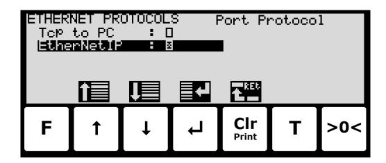
In the **ETHERNET PROTOCOLS** screen the 'EtherNetIP' parameter is selected using the cursor, and is pressed to enable or disable the Ethernet-IP protocol. A **X** in the corresponding box indicates the protocol is enabled.
