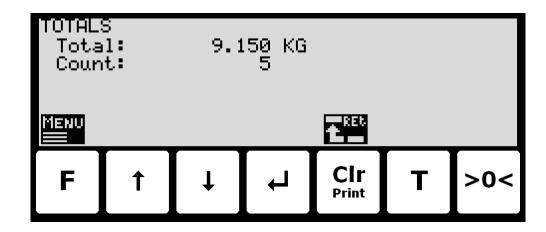
In this screen the totals are shown. Whenever a registration is performed the total weight is updated with the registered amount and the total count is incremented.
