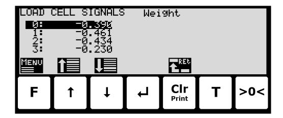
Three different readings can be selected from the LOAD CELL SIGNALS menu:
