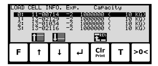
On each line for each load cell the serial number, exponent and capacity as well as in parenthesis the capacity converted to an appropriate unit depending on the exponent is shown.
