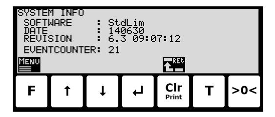
The **SETUP** screen also shows the software version (software name, date and revision):
