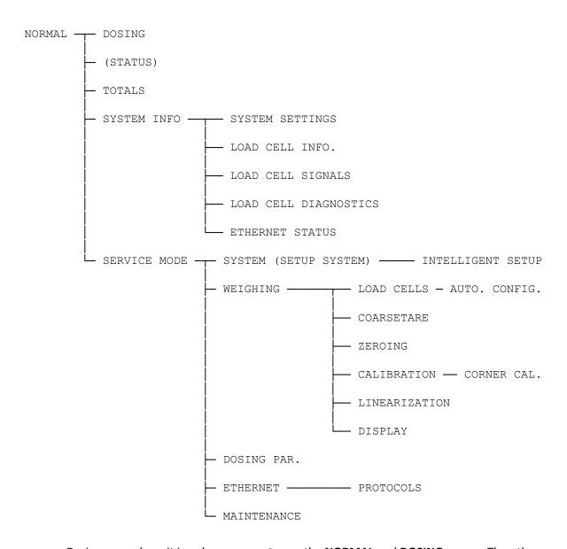
During normal use it is only necessary to use the **NORMAL** and **DOSING** screen. The other screens are used during installation and calibration.
