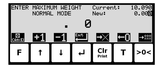
The actual parameter changed is indicated in the upper left part of the display. The current parameter value and the currently entered value is shown in the upper right part of the display. The currently entered value is also shown in the middle of the display in large font.
