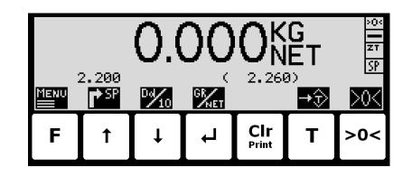
In the SETUP SYSTEM screen, change the High res. mode parameter to ENABLED (this can only be done when parameters are unlocked). Now when pressing ↓ in the NORMAL screen high resolution mode will be selected until ↓ is pressed again. The symbol above ↓ will flash while high resolution is active.
