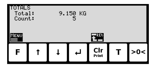
In this screen the totals are shown. Whenever a registration is performed the total weight is updated with the registered amount and the total count is incremented.
