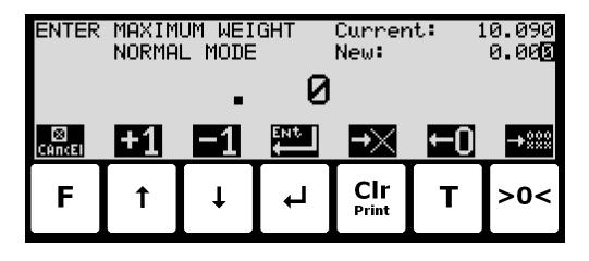
The actual parameter changed is indicated in the upper left part of the display. The current parameter value and the currently entered value is shown in the upper right part of the display. The currently entered value is also shown in the middle of the display in large font.
