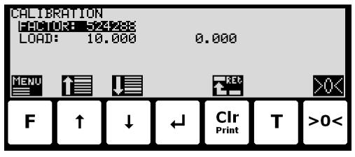
In this screen calibration parameters such as calibration factor, calibration load (to the left) and actual gross weight (to the right) are shown and can be changed. This makes it possible to calibrate the system. From the **CALIBRATE** menu it is possible to select the **CORNER CALI-BRATION** screen for corner calibration of the system. A cursor (inverted text) indicates the currently selected parameter.
