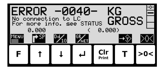
The weight indication normally shown in large types is replaced by an error code with a corresponding description and reference to the **STATUS** screen, where the error code is elaborated and possible tips to how the individual error codes can be solved are given.
