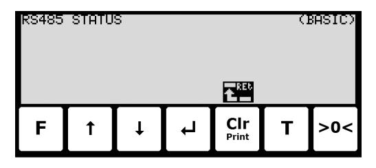
For the BASIC RS485 protocol the RS485 STATUS screen will be blank (no data is shown).
