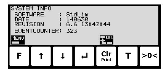
The **SETUP** screen also shows the software version (software name, date and revision):
