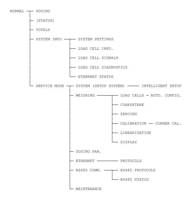
During normal use it is only necessary to use the **NORMAL** and **DOSING** screen. The other screens are used during installation and calibration.
