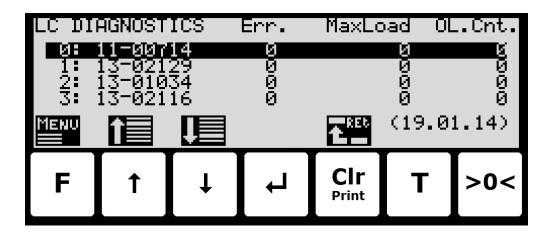
On each line for each load cell the serial number, number of detected errors (Err.), the maximum load measured on the load cell (MaxLoad) and the number of times the load cell has been overloaded (OL.Cnt.). All these numbers apply since the last reset of diagnostics data, which took place on the date shown in parenthesis in the lower right corner (YY.MM.DD).
