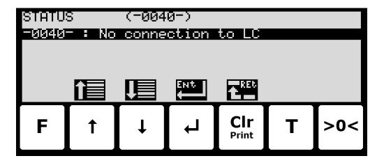
**Please notice:** Depending on the load cell protocol, a given error may result in multiple error codes at the same time. These error codes will be logical OR'ed together, and the resulting error code shown in the **NORMAL** screen is also shown in the top line of this screen.
