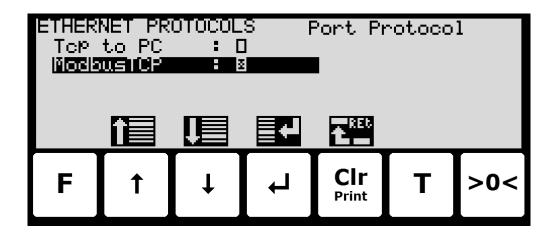
In the **ETHERNET PROTOCOLS** screen the 'ModbusTCP' parameter is selected using the cursor, and is pressed to enable or disable the Modbus TCP protocol. A **X** in the corresponding box indicates the protocol is enabled. From the appearing menu it is also possible to switch to the **MODBUS TCP DATA** screen.
