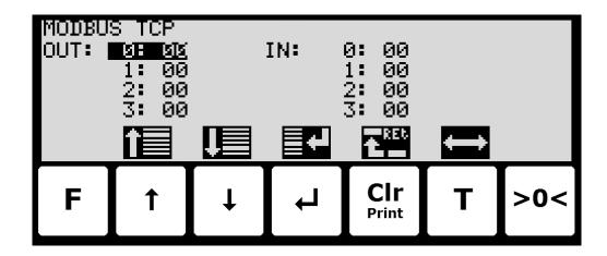
This screen will show the data sent to the Modbus TCP master (*OUT*) and the data received from the Modbus TCP master (*IN*).
