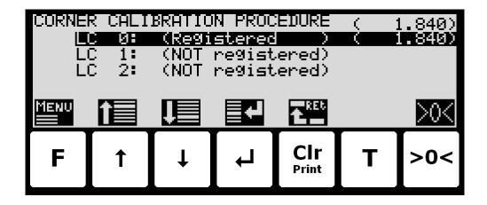
In this screen a line for each load cell will be shown indicating "NOT registered". Once the signal resulting from a given load placed above a load cell is registered this indication will change to "Registered" followed by the registered load for this load cell/corner. The actual gross weight is shown in the upper right corner.
