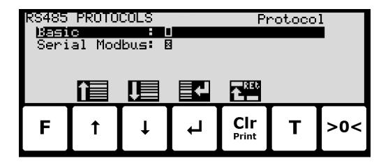
In the **RS485 PROTOCOLS** screen the 'Serial Modbus' parameter is selected using the cursor, and is pressed to enable or disable the Serial Modbus protocol. An **X** in the corresponding box indicates the protocol is enabled.
